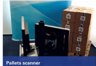
For fixed installation in the goods receipt. Captures all labels on pallet units, reads barcodes and sends information to ERP and traceability.
